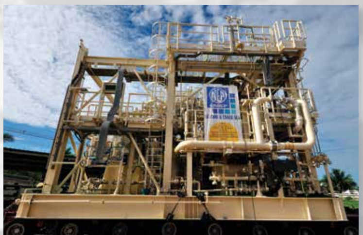
NEA compressor model: 3SVL250hs - three stage, lubricated, 4-throw, horizontal Application: Offshore Vapor Recovery
