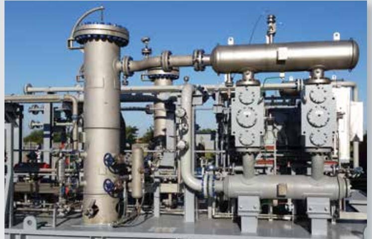
NEA compressor model: 3SVL320hs - three stage, lubricated, 4-throw, horizontal Application: CO 2 Injection for EOR
