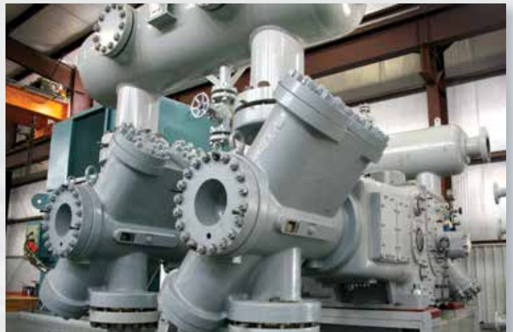
NEA compressor model: 1SVL250hs - single stage, lubricated, 4-throw, horizontal Application: Fuel Gas Booster
