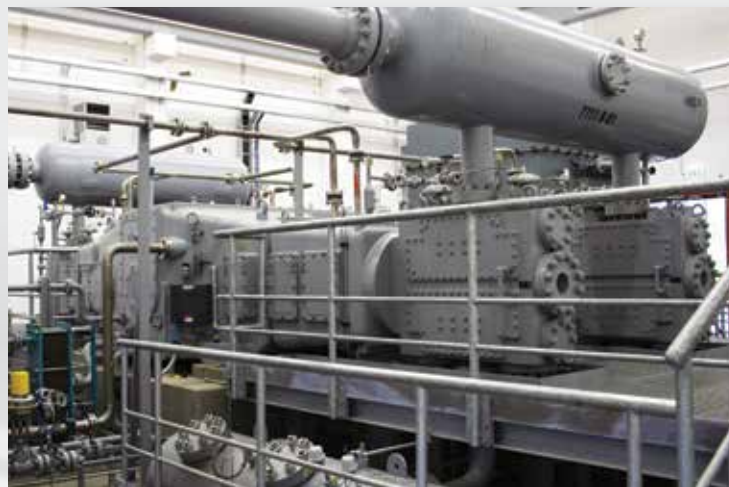
NEA compressor model: 2SVL700hs - two stage, lubricated, 4-throw, horizontal Application: Gas Storage and Withdrawal
